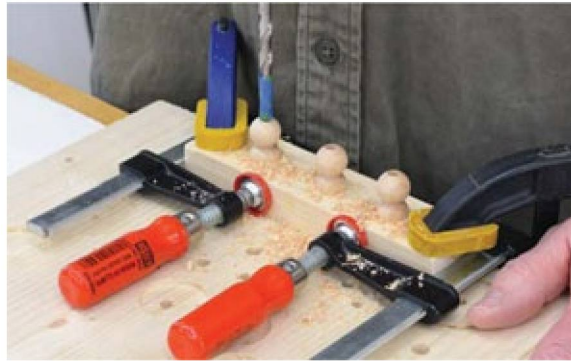
Photo 9 Secure the wooden players in the drilling jig, then drill a \frac{1}{4} " hole into the center of the tops.
