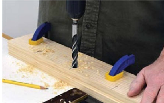
Photo 2 Measure and mark carefully, then drill the rod holes at the top of the game side pieces.
