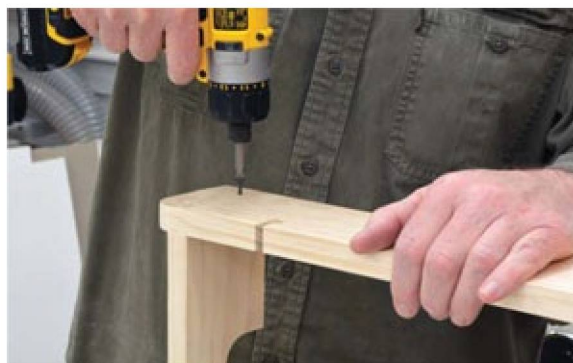
Photo 5 Reinforce the assembly by countersinking pilot holes and driving in 1-⅝” screws.
