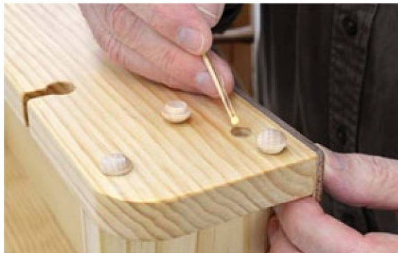
Photo 8 Put just a dab of glue around the edges of the countersinks, then tap in wooden button plugs.
