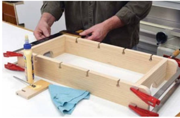
Photo 4 Apply glue to the ends of the goal sides and clamp the assembly until dry.
