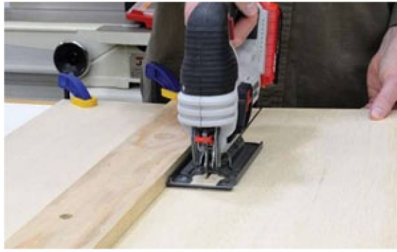
Photo 6 Cut the box bottom with a jigsaw. A clamped-on guide ensures a straight cut.
