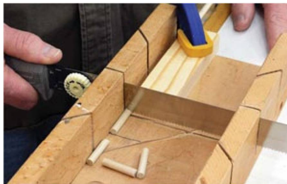
Photo 11 A pencil mark on your miter gauge makes it easy to cut several dowels the same length.
