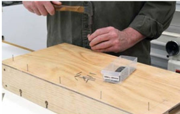
Photo 7 Apply glue to the bottom edges of the game box, then nail the bottom into place. Be sure to set the nails just below the surface.
