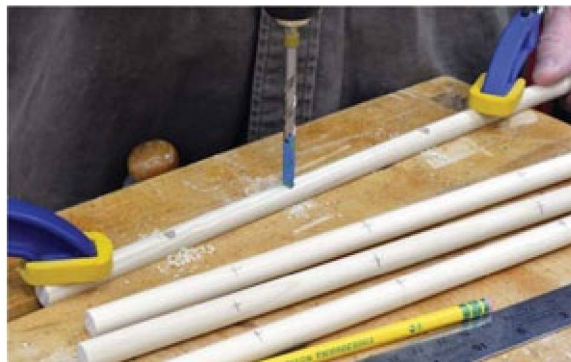
Photo 10 Clamp the control rod dowels onto a partially opened vise for drilling the player mounting holes.
