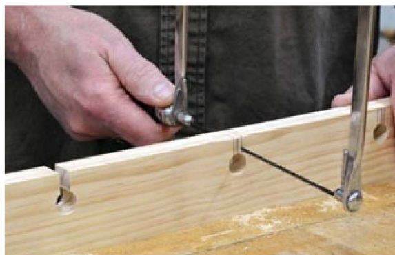
Photo 3 Create a keyhole by cutting down to the rod hole with a coping saw.
