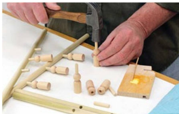
Photo 12 Put a bit of glue into the hole atop the players, and tap the mounting dowels into place.
