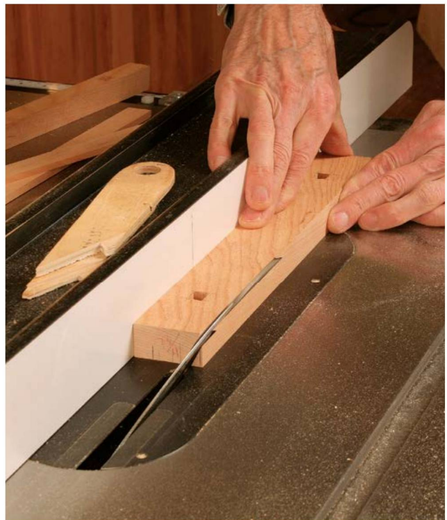
Bevels lighten the look. Becksvoort rips a bevel down the length of the top and bottom, refining the look.
