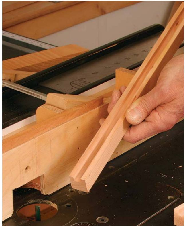
Through-grooves on the sides. With a straight bit on the router table, run through-grooves on the two side pieces.
