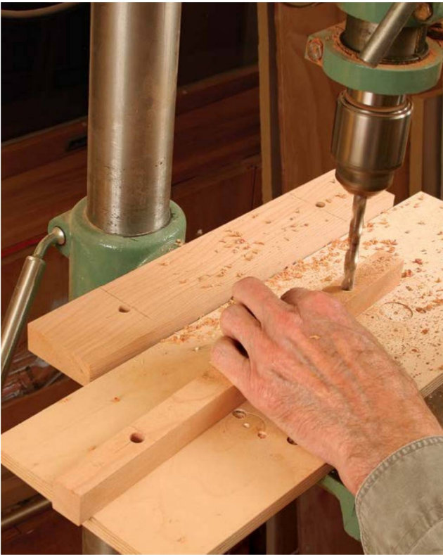
Start on the drill press. Drill through the top and bottom, centering the mortise holes in the stock.
