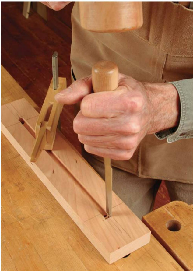
Chisel the mortises square. Now square up the mortise holes all the way through the top and bottom pieces.
