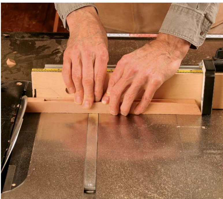
Angle the ends, too. With the tablesaw blade still tilted from the bevel, use a miter sled and cut angles on the ends of the top and bottom.
